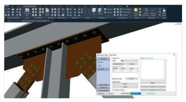
Built-in steel connection design engine.
