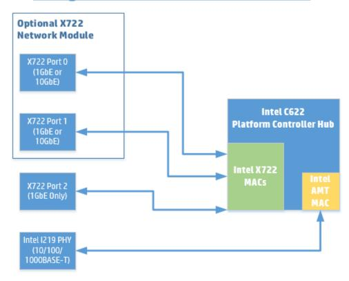
Note: When an optional X722 network module is not installed in the system, a "dummy" port is enumerated as Function O of the Intel X722 MACs, which allows for the X722 Port 2 on the Motherboard to enumerate.
